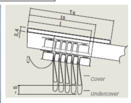
To create a nice atmospheres with wall Pergola® Awnings, it is possible to apply an "Undercover" installed under the ribs. Please note fabric will hang lower than top Vinyl cover. This undercover will be slightly narrower than the top cover by at least 4" / 10 cm per side to prevent water from going up along the PVC flap and wet the fabric of the under cover (Solid 60" fabric colors only).
