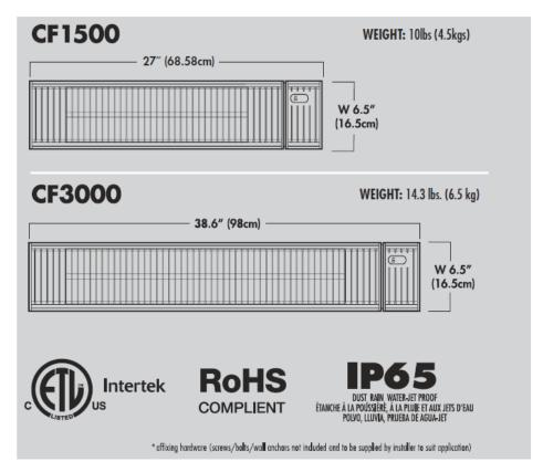
The AURA heaters is a more economical heater that simply plugs in to an outlet (110 volt version). This heater does not require a control box. The remote control is included in the price. Simply aim the remote towards the heater and you can custom set the heat from 1 - 6 on heat scale.
